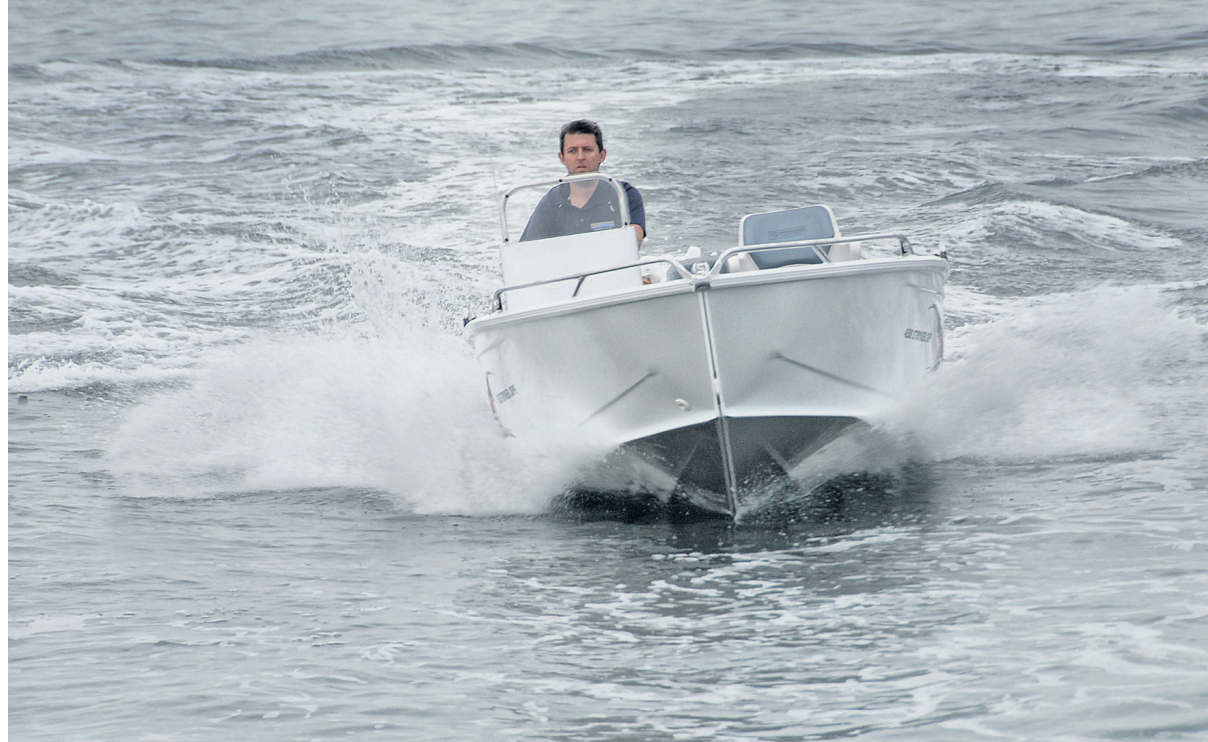
This image gives an insight into the way displaced water is pushed away from the Stryker's bow at speed.
